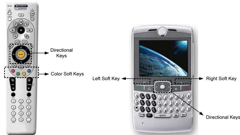
**Figure 3.** Examples of directional keys and soft keys
