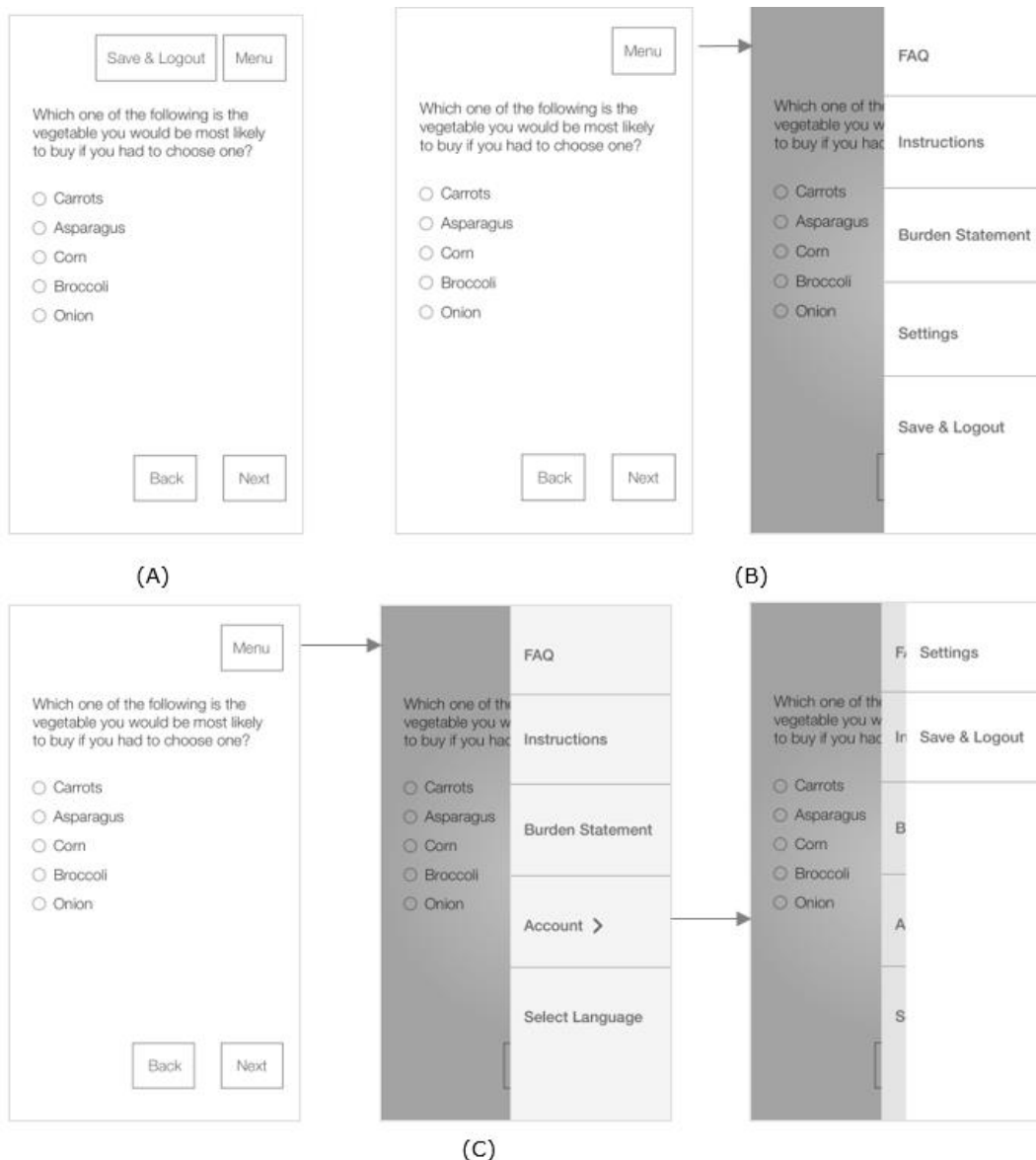
Figure 2. Placement of logout button: (A) on-screen placement, (B) main menu placement, and (C) submenu placement.
