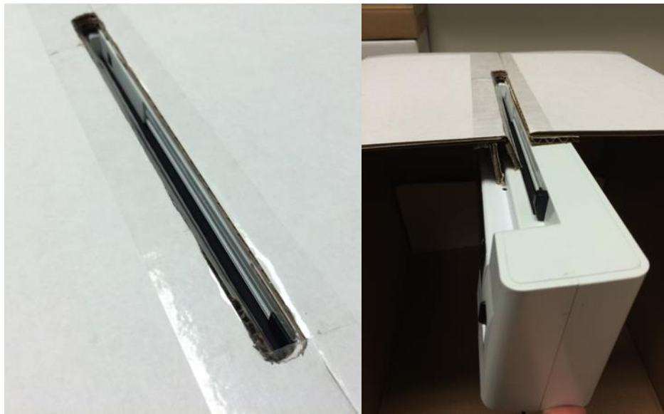
Figure 3. Detail of installed scanner and slot, user perspective and cutaway.
