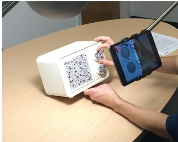
**Figure 3.** Physical model and markers enabling a TAR representation of the Sunbeam heater.
