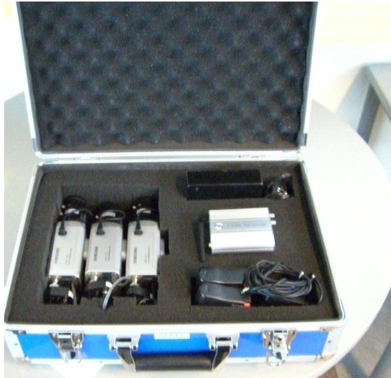
Figure 5. The whole kit fits into two aluminum cases that can be taken to the site of study. This case includes environmental cameras; the other kit contains the user-worn components.
