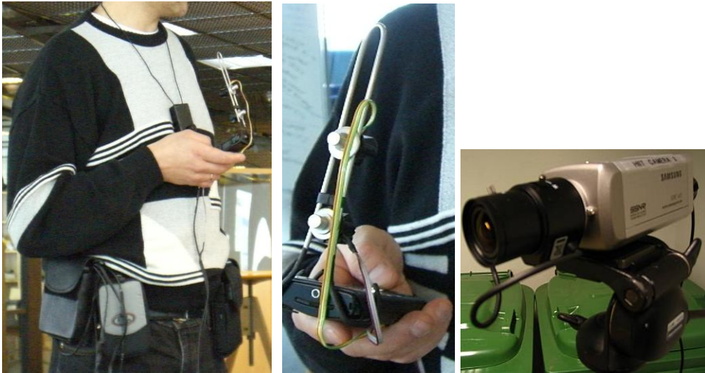
Figure 2. From left to right: All non-camera equipment attaches to a black leather belt worn by the user. In this setup the front camera is in a small black box (a necklace). (b) A lightweight pole attachable to almost any mobile device can host two minicameras; one camera capturing the face of the user, the other camera capturing the events on the display and keyboard. (c) Environmental cameras allow for higher quality third-person views. The receiver switches to the nearest camera automatically based on signal strength.
