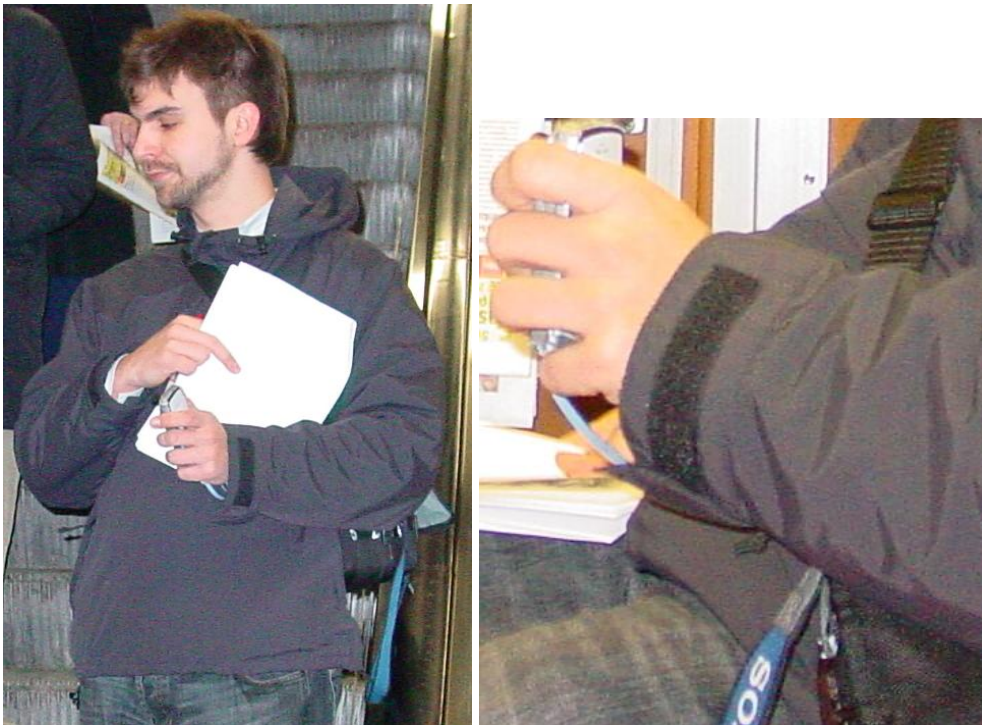
Figure 4. One of the earlier setups had the moderator-controlled camera built in a fake shell of a mobile phone. The wire goes through the sleeve to a recorder on the waist. This solution allows for quiet, non-visible recording in public places.
