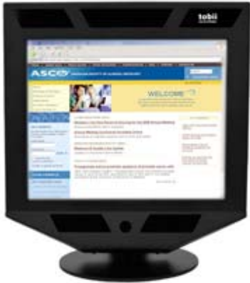
Figure 3. Tobii 1750 binocular remote eye tracker with sampling rate of 50Hz and 0.5° spatial resolution. The tracking hardware is fully integrated into the monitor and, by being almost invisible to the users, has little impact on the ecological validity of the studies.
